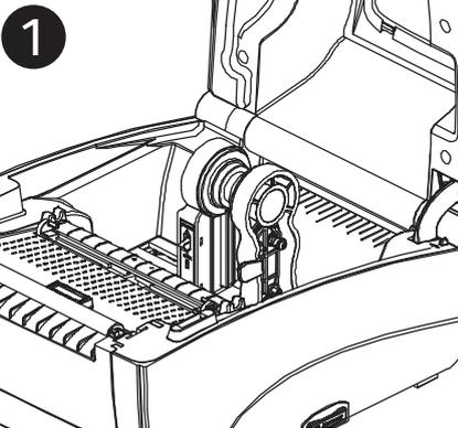
**1** Open the upper printer cover by pulling the levers on each side forwards, then raise the cover as far as it will go.
