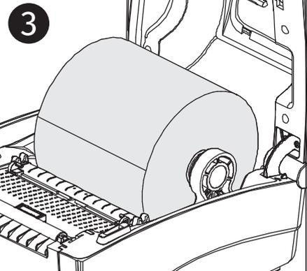
**3** Position the roll between the mounts and ensure that the bearings engage with the roll core. Secure the roll by pressing down on the media holder lock.
