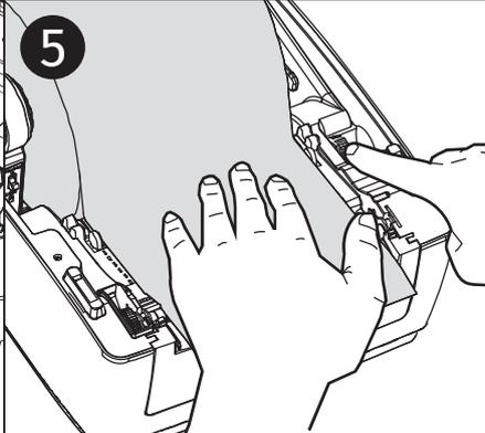
**5** Adjust the media guide width by rotating the media guide adjustment knob.
