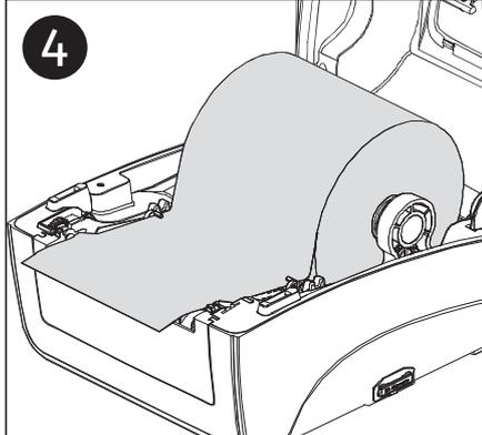
**4** Take the paper, with the printable side facing up, and pull it up through the media sensor, then place the front edge onto the cylinder.
